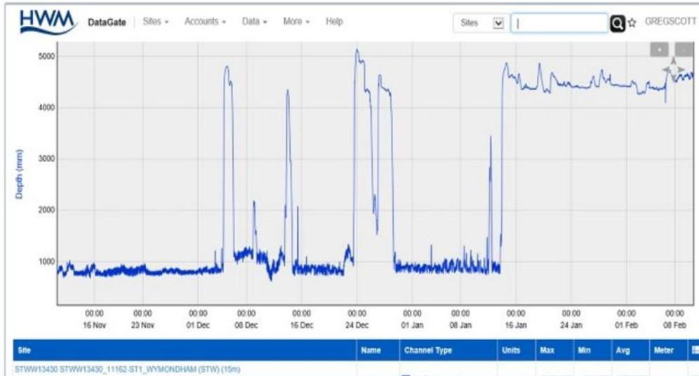
*Telemetry data shown constant flow since 14<sup>th</sup> January, highly likely potential severe infiltration into the sewer network predominantly from the brook and infiltration of the sewerage network.*
